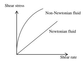
The viscosity of the fluid is defined as the ratio of the shear stress and shear rate. Thus the slope of the relation between shear-stress and shear-rate gives the viscosity  $(\eta)$ . If the plot between shear-stress and shear-rate is a straight line, the fluid is Newtonian, otherwise, it is non-Newtonian.
